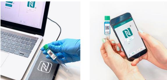
TubeSense® is prepared for dual frequency tag support (UHF RFID and NFC) and blockchain integration. This provides end-to-end visibility of shipments and products throughout the complete supply chain. If required, the TubeSense® logging devices can be equipped with additional light and shock sensors when needed for specific applications.
